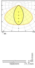
Specifications Ledvance LED Trunking Trusys Flex Clear Steel White 50W 8600lm 60D - 840 Cool White | Emergency 3H
